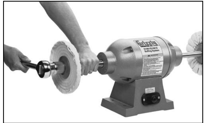
Figure 4. Buffing wheel loosening/tightening procedure.
